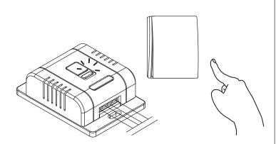
While the indicator on receiver flashes, press the Kinetic switch ONCE to complete the pairing.
