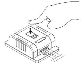
Press the Pairing Key for 10-12s, untill the Red indicator changes into Blue light.
